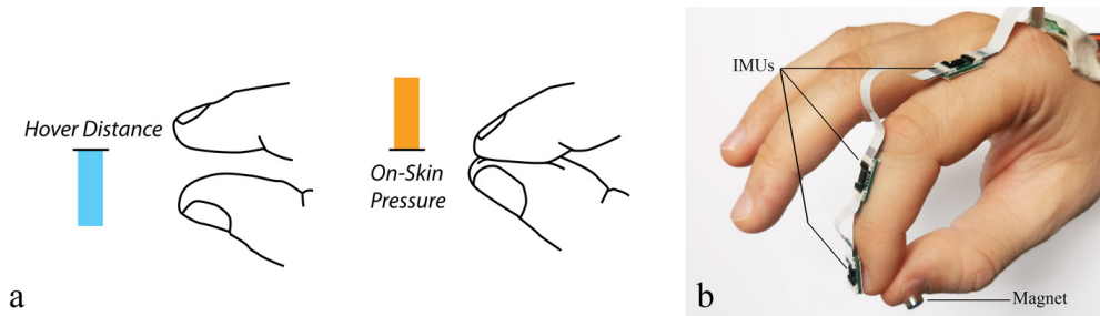
Figure 1: a) MicroPress leverages depth for thumb-to-finger interactions by enabling real-time hover and pressure input. b) It relies on IMU sensors placed on the index finger's, and a magnet placed on the thumb.
