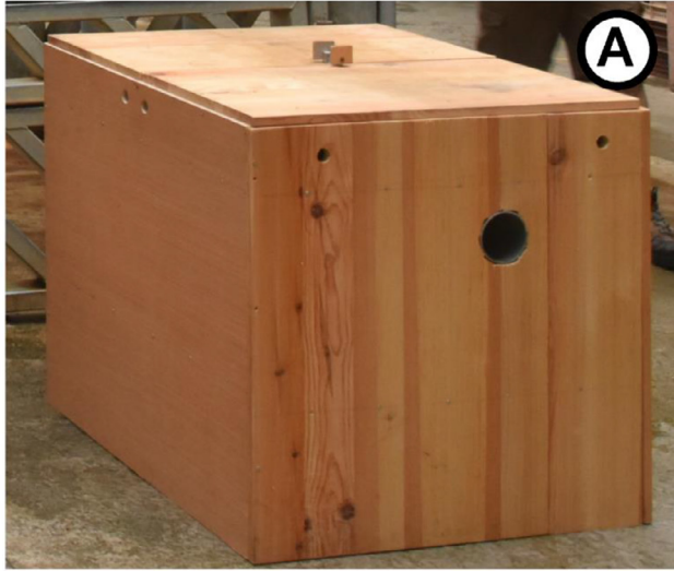
Fig. 2. A Photo of the wooden boxe seen from behind with the opening for recharging the apples; B Photo of Micro Load Cell (0-50kg) - CZL635 (Phidgets Inc., Canada) [15].
