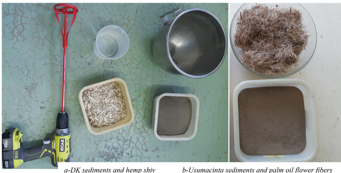
Fig. 3. Dunkirk sediments and hemp shiv (a), Usumacinta River sediments and palm oil flower fibers (b).
