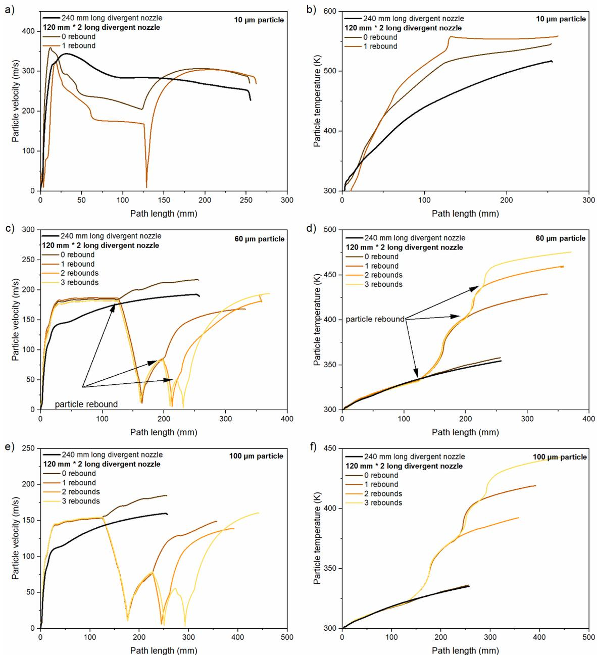
Figure 9: Evolution of the particle velocity and temperature along the nozzle path for a,b) 10  $\mu\text{m}$  particles, c,d) 60  $\mu\text{m}$  particles, and e,f) 100  $\mu\text{m}$  particles in function of the number of rebound. Comparison of the particle thermomechanical history between the 240 mm long divergent nozzle and the 120 mm  $\times$  2 long divergent nozzles.
