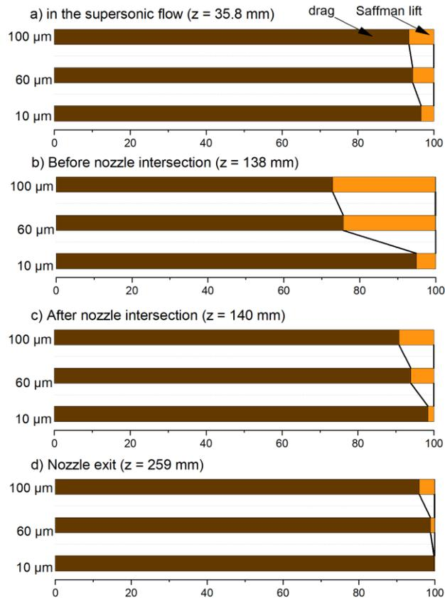
Figure 8: Force balance acting on the particle at different locations of the 120 mm  $\times$  2 long nozzle: a) in the supersonic flow, b) before the intersection between the two nozzle sections, c) after the intersection between the two nozzle sections, and d) at the nozzle exit. Thermophoretic forces and gravity are neglectable in front of drag and Saffman lift forces.
