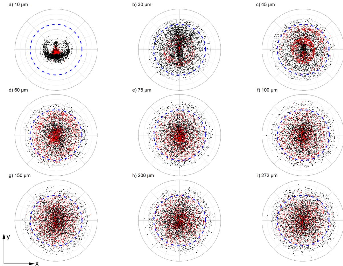
Figure 13: Repartition on the substrate of the rebounded particles (in red) and non-rebounded particles (in black) sprayed with the 120 mm  $\times$  2 long divergent nozzle for different particle sizes. The diameter of the blue dashed circle is equal to 5 mm, i.e., the nozzle exit diameter.
