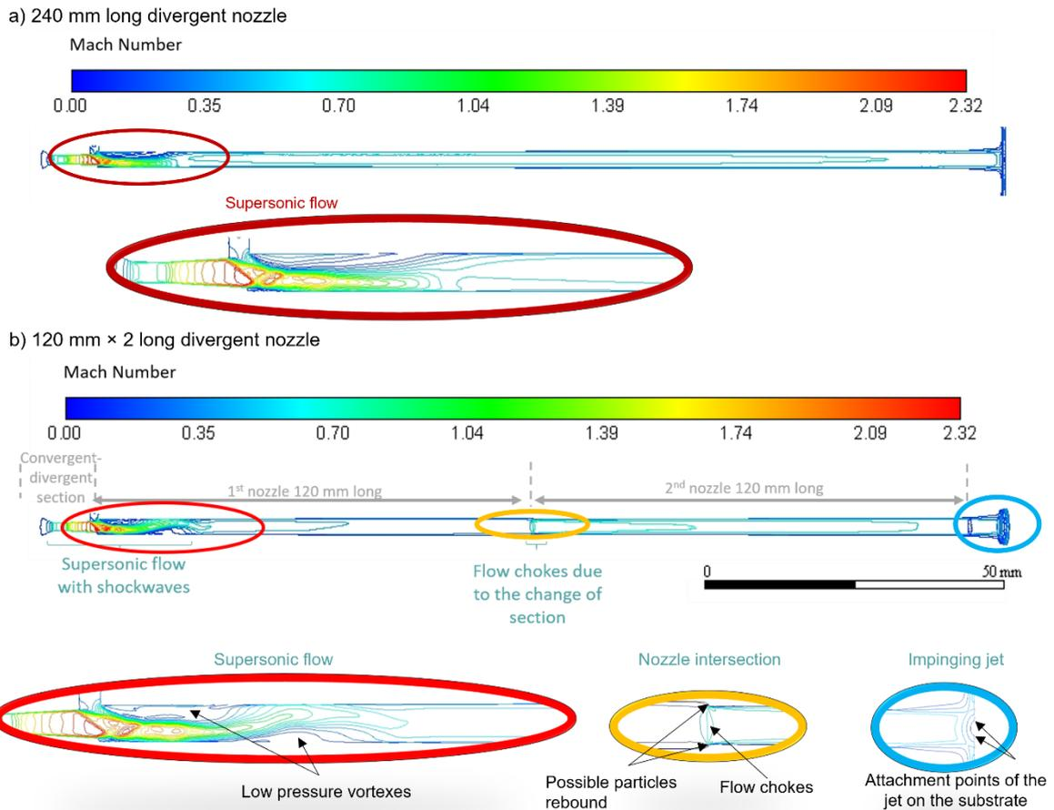
Figure 4: Evolution of the Mach Number along the nozzle for a) 240 mm long divergent nozzle and b) 120 mm x 2 long divergent nozzle. For the 120 mm x 2 long divergent nozzle, two large vortices are observed close to the particle inlet. In addition, at the intersection between the two nozzles, flow chokes due to the reduction of section.
