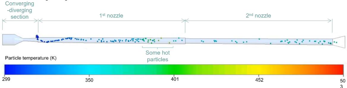
Figure 6: Evolution of the particles' trajectories along the a) 240 mm long nozzle and b) 120 mm × 2 long nozzle. For the 120 mm × 2 long nozzle, at their entrance into the nozzle, all particles follow the same path. At the intersection between the two nozzle sections, some particles are rebounding inside the nozzle leading them to go upstream and reaching a higher temperature. All particles have a diameter of 60  $\mu\text{m}$ .
