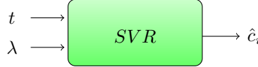
Figure 1: A SVR takes as input a time step t and one or several parameters \lambda . It outputs a prediction \hat{c}_i , corresponding to the i -th coefficient on the reduced space, i = 1 \dots r .
