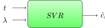
Figure 1: A SVR takes as input a time step t and one or several parameters \lambda . It outputs a prediction \hat{c}_i , corresponding to the i -th coefficient on the reduced space, i = 1 \dots r .
