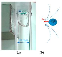
**Figure 1.** (a): Liquid rising in a bottle containing the paramagnetic solution (Tb(NO<sub>3</sub>)<sub>3</sub>, 1M), whose surface is deformed due to the application of an inhomogeneous magnetic field (photograph). The whole solution is drawn to the pole of a 2T magnet. (b): The magnetic gradient force ( $F_{\nabla}$ ) acts on the paramagnetic ions which drain the solution until equilibrating the forces by the weight of the attracted volume.
