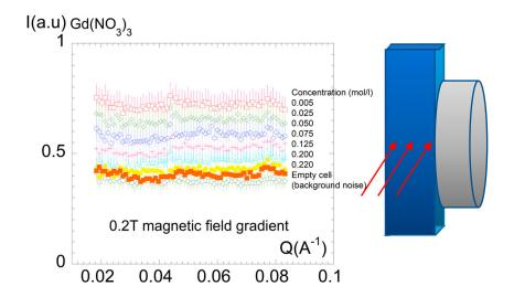
**Figure 5.** Neutron scattering intensity measured at small-angle scattering on a series of different concentrations of solutions of Gd(NO<sub>3</sub>)<sub>3</sub> solubilized in deuterated water (PA20 spectrometer). The liquid container (in blue) was placed in contact to a pole of 0.2T magnetic field, as illustrated in the scheme at the right of the figure, to submit the paramagnetic liquid to a field gradient. Room temperature measurements.
