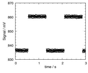
FIG. 7. Detector photodiode voltage sampled by the AD converter at a rate of 860 samples/s while the red LED power is modulated by 0.4%. The effective sample rate was 323 samples/s. No transitions between the levels can be observed, so the time response of the detector photodiode is better than 3.1 ms.
