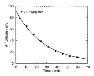
FIG. 16. Decrease in amplitude of the marathon curves in Figure 15 with increasing time agrees very well with an exponential decay.
