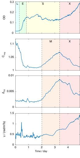
FIG. 14. Four bacteria suspension parameters measured over a span of five days: (i) optical density (OD), (ii)  $C_{\text{mag}}$ , which quantifies the ratio of magnetic to nonmagnetic bacteria, (iii)  $\Delta_{\rm OD}$ , which quantifies the amount of magnetic bacteria, and (iv)  $\gamma$ , which quantifies how strongly the bacteria respond to magnetic fields. The following phases can be identified: lag L, exponential E, stationary S, magnetic growth M, and an undefined phase X.
