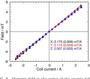
FIG. 9. Magnetic field in the center of the cuvette holder as a function of average coil current. Fields in x, y and zdirection with a field-to-current ratio of 2.175(9), 2.113(3) and  $2.007(3) \,\mathrm{mT/A}$ , respectively.
