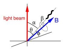
FIG. 2. Definitions of various angles. In our MagOD system, we set the angle  $\theta$  between the light path and the magnetic field B. The bacteria align with the direction of the field, but can deviate by a small angle  $\phi$  in a cone around the field direction described by  $\beta$ . As a result, the angle between the bacteria long axis and the light is  $\alpha$ . In case of sufficiently large fields,  $\phi=0$ ,  $\alpha=\theta$ , and  $\beta$  is irrelevant.
