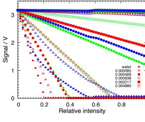
FIG. 19. Signal as a function of the LED duty cycle for the three different LED wavelengths as well as for a water reference and three different dilutions of a EMG304 magnetic nanoparticle suspension.
