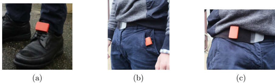
Figure 2.: Position of the wearable sensors on the body: Foot-mounted (a), in the pocket (b), waist-attached (c)
