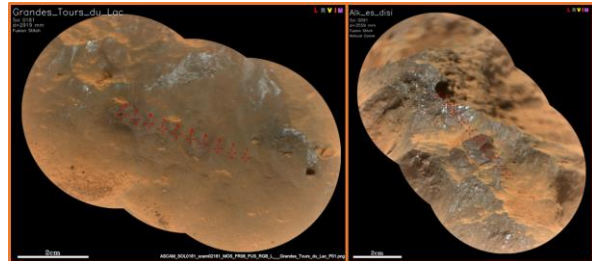
Fig. 4: Sulfate-rich coatings on targets Grandes Tours du Lac and Alk es disi.
