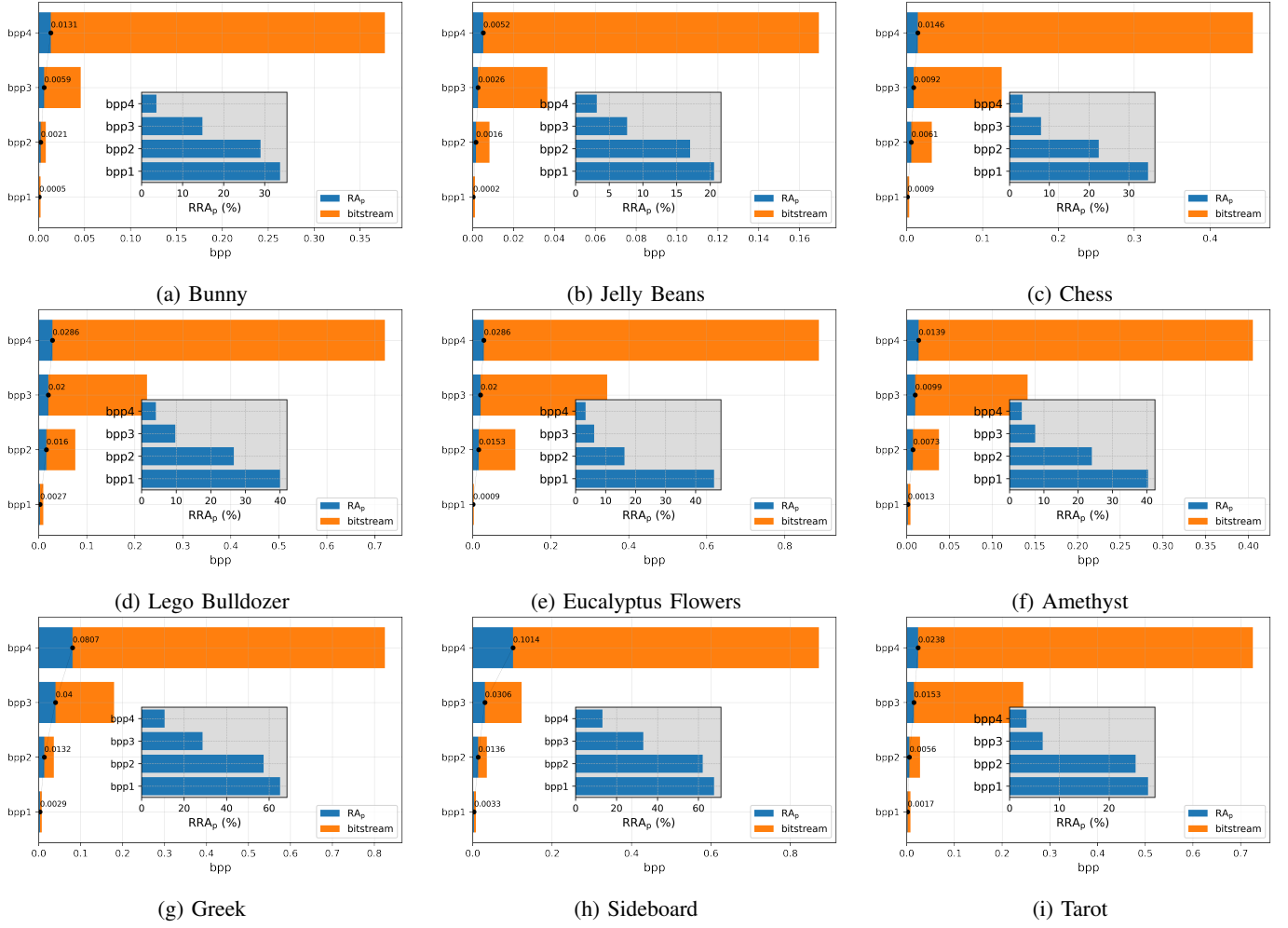
Fig. 12: RA_p and RRA_p for light field test images. RA_p denotes the maximum number of encoded bits required to access an arbitrary view at each bitstream. The embedded plots represent RRA_p , i.e., the relative number of encoded bits required to access an arbitrary view at each bitstream.
