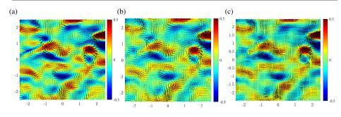
Fig. 7: Instantaneous velocity field results for the two-dimensional HITF dataset. DNS results (a), OF results (b), CC PIV results (c).
