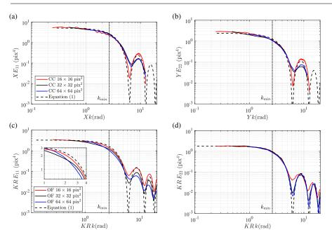
Fig. 3: Power spectra of displacements from no-motion PIV maps obtained with Cross-Correlation (with 75% overlap for CC) in (a) and (b) and Optical Flow (with an overlap of (KR-1)/KR > 93%) in (c) and (d), along the *x* direction in (a) and (c) and along the *y* direction in (b) and (d).
