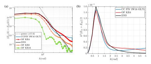
Fig. 8: (a) Velocity spectra comparison for the THIF data-set. Comparison with spectra from reference DNS data. 10 iterations and 2 pyramid levels are used for OF calculations. (b) Dissipation rate comparison for the THIF data-set. Comparison with spectra from reference DNS data.
