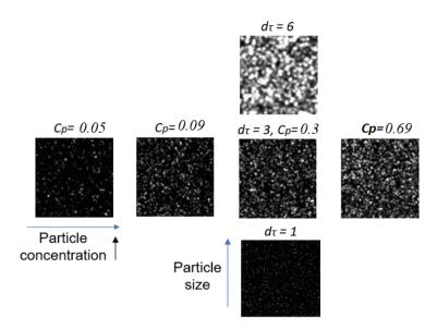
Fig. 4: Examples of synthetic particle images with increasing particle concentrations (from left to right) for a given particle diameter ( $d_{\tau} = 3 \text{ px}$ ) or with increasing particle diameters (from bottom to top) for a given concentration ( $C_p = 0.3 \text{ ppp}$ ). The size of the image is  $100 \times 100 \text{ px}^2$ .
