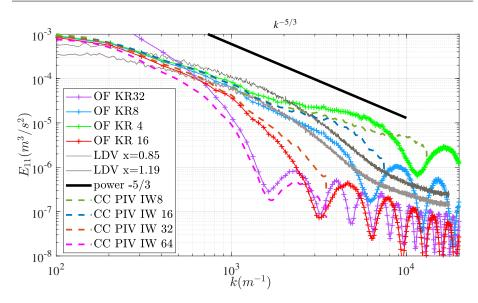
Fig. 12: Time-averaged velocity spectra of the streamwise velocity component along a streamwise profile in the centre of the velocity field, compared with LDV measurements spectra at two streamwise positions (z = 0.02 and x = 0.06 shown in Fig. 10).
