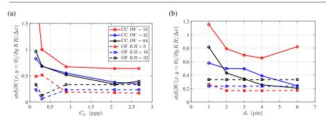
Fig. 6: Maximum of the standard deviation computed in Fig. 5(e,f) of the shear as a function of both (a) the particle concentration  $C_p$  computed for  $d_{\tau} = 3$  px and (b) the actual particle size  $d_{\tau}$  for  $C_p = 0.69$  ppp. Here the continuous lines corresponds to the results obtained with CC while dashed line correspond to OF.
