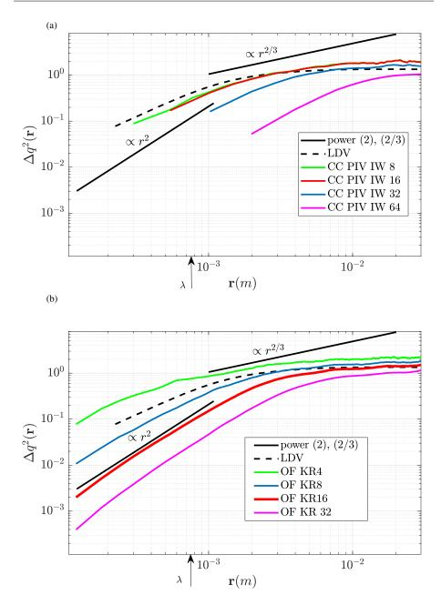
Fig. 11: Evolution of the second-order structure function with respect to the separation scale r along the normal direction to the mean flow, for CC PIV (a), OF (b) compared to LDV measurements. Results are averaged in time.
