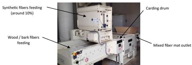
Fig. 2 Processing equipment used for 3D fiberboard formation: nap- opener or air-laid machine from Laroche
