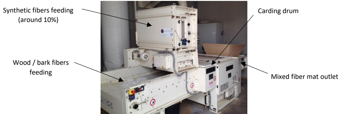
193 194 Figure 2. Processing equipment used for 3D fiberboard formation: napper opener machine from Laroche. 195 196
