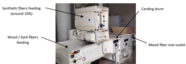
Fig. 2 Processing equipment used for 3D fiberboard formation: nap- opener or air-laid machine from Laroche
