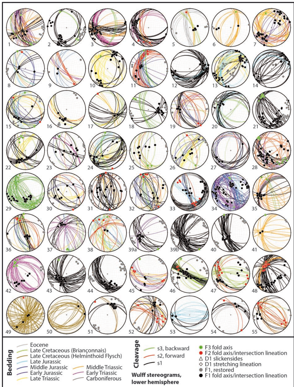
Figure 11: Microstructural data of the 55 sites (location table I) investigated in the Briançonnais/Prepiedmont zones and nearby in the Embrunais-Ubaye nappes and the Schistes Lustrés. Red and green dots represent the forward and backward late (D2) fold trends, respectively. Black dots are the early (D1) trends, and grey dots represent the latter restored from D2 deformation (where needed). The median trends at each site are reported on fig. 10.
