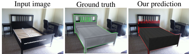
Figure 6. Inaccuracies in ground truth annotations in the Pix3D dataset. Example of an alignment with an incorrect 3D model predicted by our approach (right) that results in a lower 3D translation and focal length errors compared to the aligned ground truth 3D model (middle). This is caused by a mismatch between the bed depicted in the input image (with no mattress) and the ground truth 3D model.
