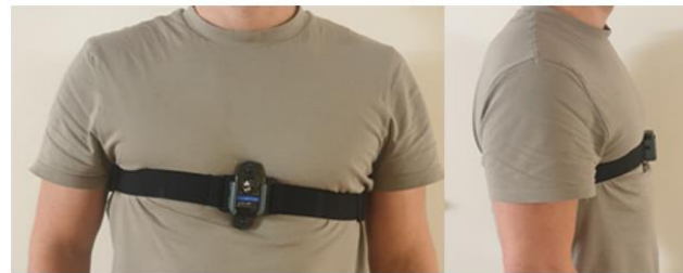
Figure 1. Placement of the inertial measurement unit on the body as described in Warmerdam et al., (2021) [31].
