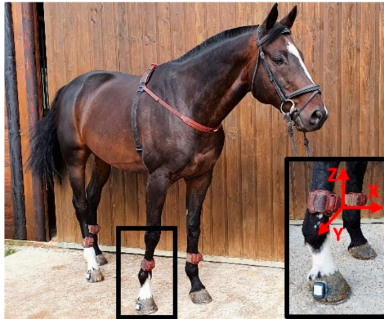
Figure 1. IMUs localization on horse: on the withers, on the four limbs, in the center of the dorsal side of the third metacarpal bone (cannon bone), and on the lateral quarter of the right front and hind hoof.
