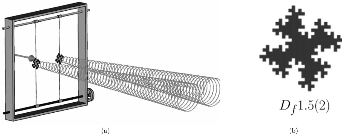
FIG. 1. (a) Sketch of the experimental wind tunnel setup; (b) Irregular plate used herein. They are the second iteration of a fractal plate with dimension  $D_f = 1.5$  and a square initial pattern, as characterised by [26].
