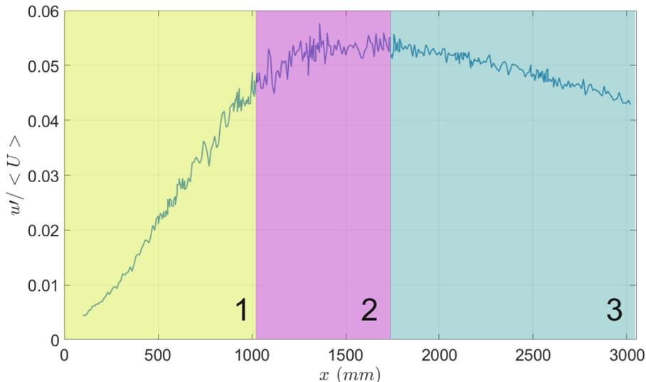
FIG. 2. Streamwise distribution of  $u'/\langle U \rangle$  for the irregular plates at  $S = 285\text{mm}$ .
