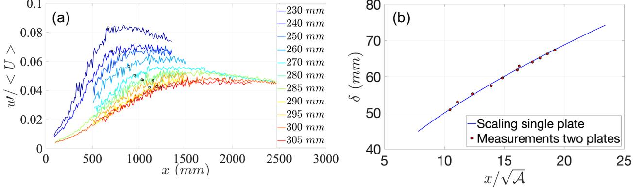
FIG. 6. (a) Streamwise profile of the velocity fluctuations for all plate separations  $S$  in table I. The black squares represent  $x_{12}$ , i.e. the  $x$ -locations of the transition between regions 1 and 2; (b) Comparison of the wake half width profile obtained for a single irregular plate by [13] (blue line) with the results obtained using equation 9 in the wake-interaction setup used here (red circles).
