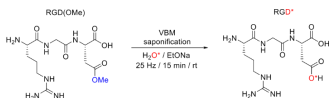
Scheme 4. Synthesis of site-selectively ^{17}\text{O} -enriched RGD* tri-peptide by VBM saponification of methyl ester protected peptide (prepared by SPPS, for synthetic details see SI). Only one oxygen is labeled per ester-derivatized carboxylic function using mechanochemistry, but globally, the labeled oxygen is distributed between both oxygen sites ( i.e. C=O* and C-O*H, 50 : 50).
