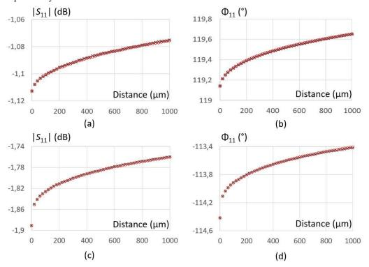
Figure 3. Amplitude and phase-shift of the reflection coefficient  $S_{11}$  as a function of the probe-metallic sample separation. (a)-(b) f = 1 GHz and (c)-(d) f = 2 GHz.
