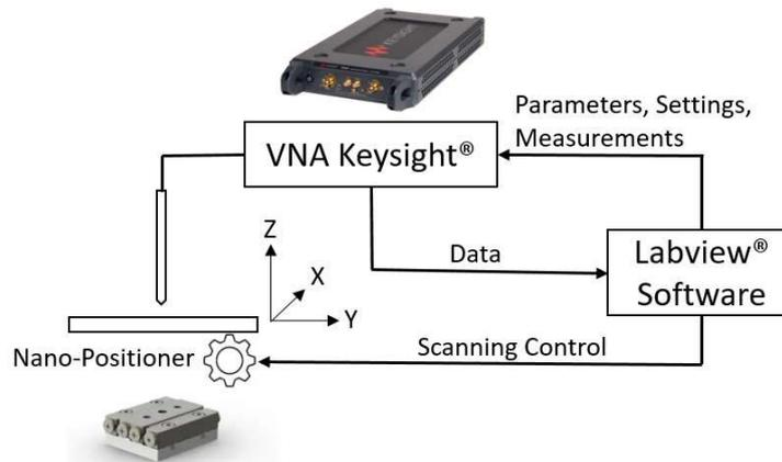
Figure 2. General overview of the proposed Nanorobotics microwave platform for liquid sensing applications.
