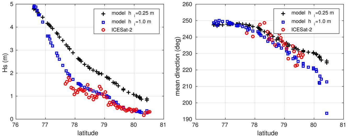
**Figure 4.** Wave heights and mean wave directions (from, nautical convention) along the ICESat-2 track at 4:00 UTC on 23 March 2019, according to two different model simulations or taken as the average of the 6 wave heights estimated for each of the six ICESat-2 laser beams.
