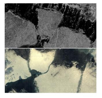
**Figure 5.** Same ice floes observed by Sentinel 1 at 9:00 UTC and Sentinel 2 at 11:07 UTC on 23 March 2019, around 78.15°N, 46.00°E. The Sentinel two image is a true color composite using bands B02, B03, and B04.
