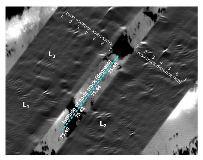
**Figure 9.** Unfolded Sentinel-3 radar backscatter from Full-Focus SAR (FF-SAR) processing using Fourier analysis to separate near-horizontal features from near-vertical features in Figure 8b, and inverse Fourier transform that generates a left-side image with near-horizontal features and a right-side image with what was near-vertical when folded to the left which now appears also near-horizontal. The background image is Sentinel-2.
