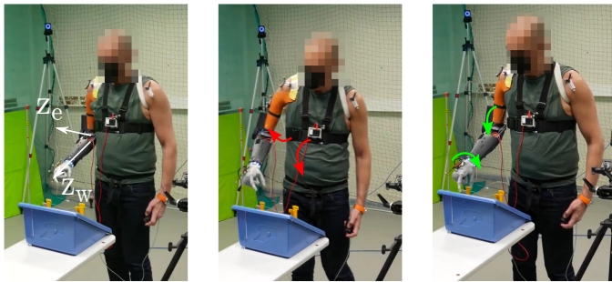
(a) The prosthesis user wants to pick the clothespin, which requires simultaneous wrist pronation (around z_w ) and elbow extension. (around z_e ). (b) With an initially still prosthesis, the user starts mobilizing task-oriented upper arm and torso compensations (in red). (c) Compensations are detected and used to generate adequate prosthesis motions (in green), which naturally leads the user to cancel compensatory motions.
