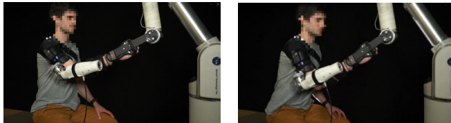
Fig. 1: A subject equipped with a robotized elbow, and having his wrist and hand locked, is asked to position a distal point at a given location materialized by a robot manipulator. On the left, a correct elbow positioning ( 135^\circ between the human humerus and the robotic ulna) results in a global posture that seems natural. On the right, with an erratic elbow joint position ( 90^\circ between humerus and ulna) the subject has to lean his trunk to achieve the task. This is called a body compensation .
