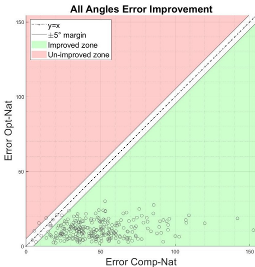
Fig. 6: Absolute error after optimization as a function of the error before optimization for the sum of the trunk, scapula, elbow and wrist angle. The dark dashed-dotted line represents the y = x axis, and the thin black lines the \pm 5^\circ margin of our estimated noise.
