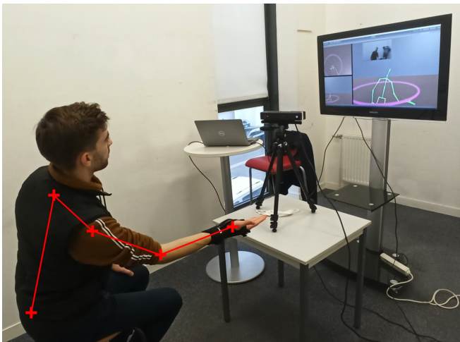
Fig. 2: View of the experimental setup used: a subject (with his measured skeleton added in red), performing a compensatory movement (while maintaining his hand position and orientation) in front of the Kinect V2; A visual interface indicates the hand position/orientation to reach and displays the subject's skeletal model, from different perspectives
