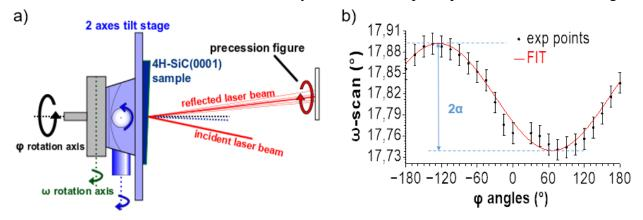
Fig. 1. (a) Scheme of the experimental setup to align the substrate's normal and the axis of the inplane rotation ( $\varphi$ -axis) of the diffractometer, (b)  $\omega$ - $\varphi$ -XRD map of the 4H-SiC(0001), measured near the (000n) reflection, with n an integer number, indicating the miscut angle  $\alpha$ .
