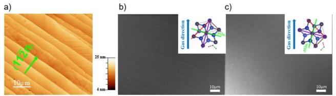
Fig. 2. (a) Topological AFM image on a sample surface that had a rotation of  $45^{\circ}$ ccw during the growth (50  $\mu$ m×50  $\mu$ m); (b) and (c) Optical microscopy (OM) images of a sample grown with the plan ( $11\overline{2}n$ ) close to perpendicular and close to parallel to the gas direction, respectively. For each OM image, the corresponding VESTA schematization is given [11].
