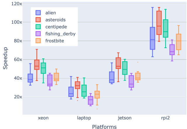
Fig. 4: Speedup in inference time of the generated code with respect to the library. Each box-plot represents the statistics for the 10 TPGs trained for a given game, and inferred on a specific platform.
