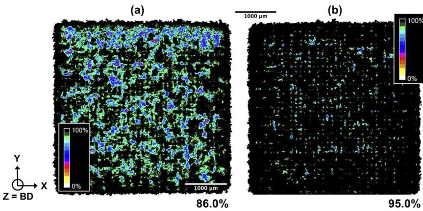
**FIG. 6.** Axial cumulative projected view of all the slices along with the height (build direction) of the sample: (a) sample 1 (75 J/m) and (b) sample 2 (100 J/m). Color code shows the local relative density: white means that a pore goes through the entire sample height while black means that the sample is locally fully dense.
