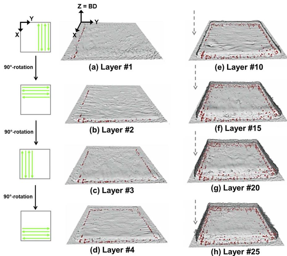
**FIG. 10.** (a)–(h) 3D rendering of sample A under fabrication at different layers. Here,  $P = 150$  W and  $v = 250$  mm/s resulting in a keyhole regime (multimedia view 10). The scanning strategy is indicated using schematics so that links between the spatial distribution of defects within the sample and the scanning strategy can be established. Pores are displayed in red. The edge of the scanned area is 4 mm. Multimedia view: <https://doi.org/10.1063/5.0090623.2>
