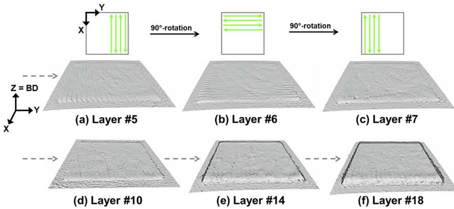
**FIG. 12.** (a)–(f) 3D rendering of sample B under fabrication at different layers. Here,  $P = 150$  W and  $v = 750$  mm/s resulting in a conduction regime (multimedia view 12). The scanning strategy is indicated using schematics. Pores are displayed in red. The edge of the scanned area is 4 mm. Multimedia view: <https://doi.org/10.1063/5.0090623.3>
