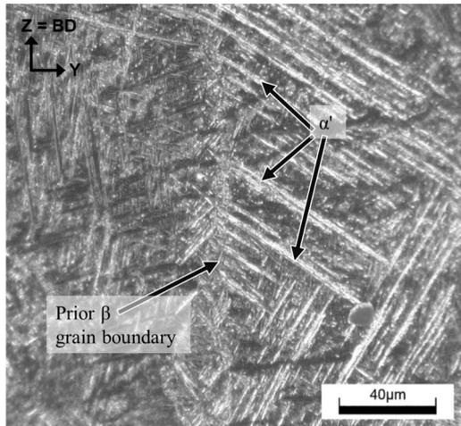
**FIG. 8.** Optical micrograph taken in sample 3 after chemical etching (Kroll reagent) revealing the presence of fully  $\alpha'$ -martensitic microstructure under the as-fabricated conditions.
