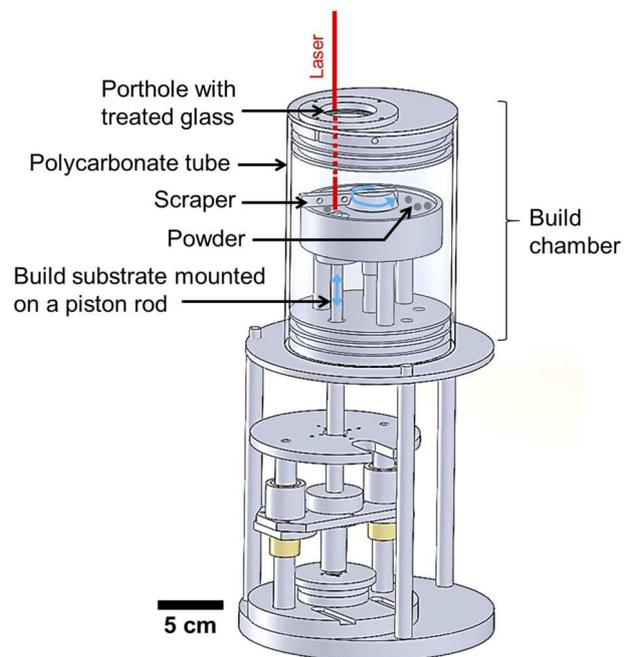
FIG. 1. 3D CAD-view of our custom-designed L-PBF replicator.
