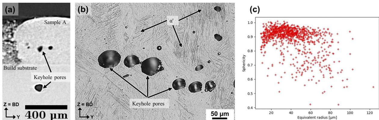
**FIG. 11.** (a) 2D cross section extracted from the edge of sample A and showing the presence of keyhole pores. (b) Optical micrograph revealing the martensitic microstructure and the presence of keyhole pores. (c) Analysis of the pore population in sample A: sphericity vs equivalent radius.
