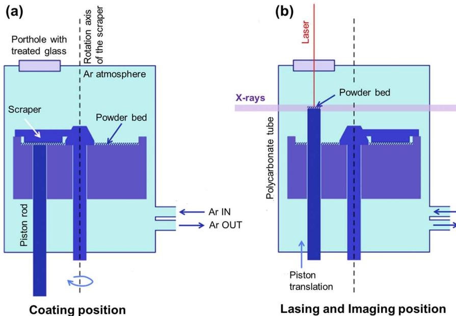
**FIG. 2.** Schematics showing the two configurations of the system: (a) coating position (piston down) and (b) lasing and imaging position (piston up).
