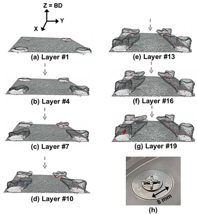
**FIG. 14.** (a)–(g) 3D rendering of the build history of the first layers of fabrication of a lattice structure unit cell (multimedia view 14). (h) Picture of the first layers of a lattice unit cell built using our miniature laser powder bed fusion. Multimedia view: <https://doi.org/10.1063/5.0090623.4>
