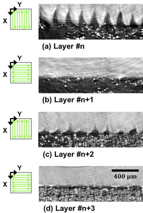
**FIG. 13.** 2D cross sections (X, Y) extracted from the reconstructed volume of sample B at a given height (Z position fixed). Four consecutive layers are shown: (a) Layer #n, (b) Layer #n + 1, (c) Layer #n + 2, and (d) Layer #n + 3. For each layer, the scanning strategy is schematically represented.
