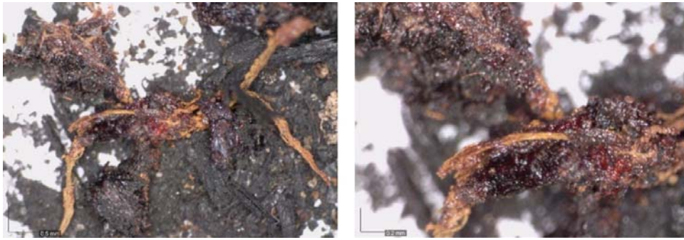
Figure 5: Detection of small fibers located on the puddening of the ring (Photo: Author).
