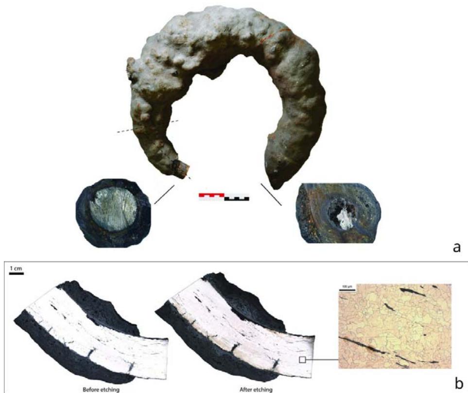
Figure 6 a): The collected anchor ring and visualization of the state of the metal corrosion at both cut ends. b): Cross-section of the sample and metallographic observation that highlight the ferritic nature of the ring.
