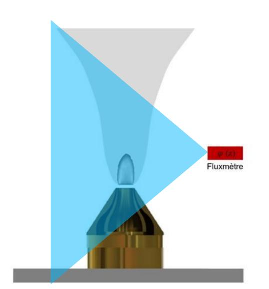
Solid angle visualization of the fluxmeter
