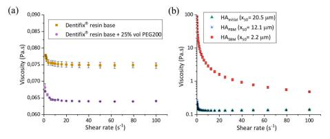
**Fig. 7.** (a) The flow data for Dentifix® resin base with and without the addition of 25% vol. of PEG200 as diluent. (b) The flow data for photocurable suspensions filled a 20% vol. with different HA powders (HA<sub>Initial</sub>, HA<sub>PBM</sub>, HA<sub>SBM</sub>) with different median particle sizes (HA<sub>Initial</sub> and HA<sub>PBM</sub> show very close viscosities).
