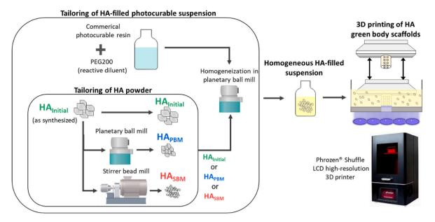
Fig. 1. HA-filled photocurable slurry preparation process.
