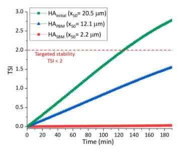
Fig. 9. TSI values of HA-filled suspensions as a function of time (T = 25  $^{\circ}$ C).
