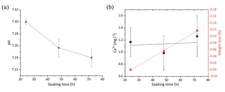
Fig. 19. (a) TRIS solution pH evolution, (b)  $Ca^{2+}$  ion release, and scaffold weight loss evolution as a function of the sintered HA scaffold soaking time. (N = 3).
