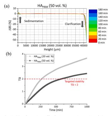
Fig. 11. (a) Backscattering profile of HA<sub>PBM</sub> suspension at 50% vol. (T = 25 °C). (b) TSI values of HA<sub>PBM</sub> filled suspensions at different concentrations as a function of time (T = 25 °C).
