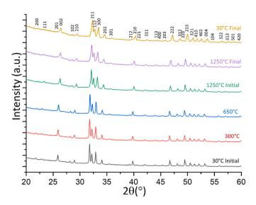
**Fig. 12.** In-situ XRD diffractograms of the HA scaffolds during the debindingsintering process at different temperatures. All the diffraction peaks correspond to stoichiometric hydroxyapatite (JCPDS 00-009-0432).
