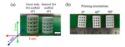
**Fig. 15.** Visual examination of HA parts: (a) comparison between green body and sintered HA scaffolds (including axes arrows), (b) comparison between sintered HA scaffolds printed at three different orientations ( $0^\circ$ , 45°, and 90°). (For interpretation of the references to colour in this figure legend, the reader is referred to the Web version of this article.)
