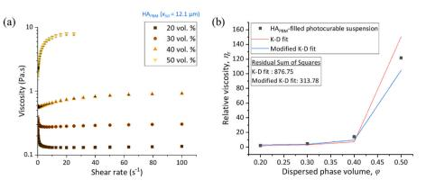
**Fig. 10.** (a) The viscosity-shear rate curves obtained for several HA-filled suspensions containing different  $HA_{PBM}$  concentrations. (b) Krieger-Dougherty (red line) and modified Krieger-Dougherty (blue line) fits for relative viscosities in  $HA_{PBM}$ -filled suspensions. (For interpretation of the references to colour in this figure legend, the reader is referred to the Web version of this article.)
