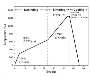
Fig. 4. Programmed temperature pattern for the debinding-sintering process of HA scaffolds.
