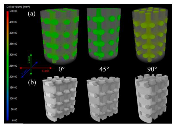
**Fig. 18.** Visualization obtained using X-ray micro-computed tomography of the three kinds of HA scaffolds ( $0^{\circ}$ ,  $45^{\circ}$ , and  $90^{\circ}$ ) produced by MSLA after the debindingsintering treatment. (a) The pore distribution of HA scaffolds with previously modelled interconnected macroporosity and circular overtures of 1000 µm in the three directions. (b) Cross-section views of HA scaffolds in X–Y, and Y-Z planes.
