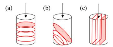
Fig. 5. Direction of loading (black arrows) to printing orientation in compressive testing. (a)  $0^{\circ}$ , (b)  $45^{\circ}$ , and (c)  $90^{\circ}$ .
