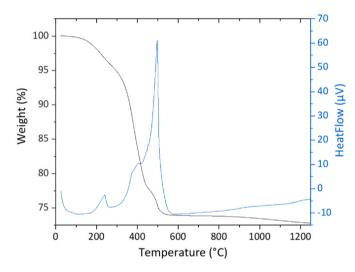
**Fig. 13.** Differential scanning calorimetry (DSC) and thermogravimetric analysis (TGA) of HA green body scaffold. (For interpretation of the references to colour in this figure legend, the reader is referred to the Web version of this article.)
