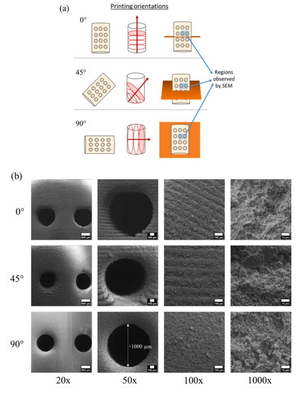
Fig. 16. (a) Three different schematic representations of the three printing orientations employed. (b) SEM micrographs at different magnifications of the HA scaffolds (X, Z plane) printed at three different orientations.
