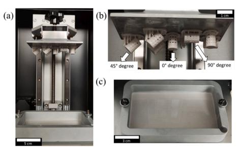
Fig. 3. (a) General view of the MSLA process, (b) printing platform with HA scaffolds with three different printing orientations, and (c) HA-filled slurry container.
