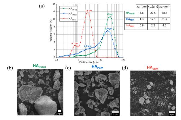
Fig. 6. (a) PSD and SEM micrographs of HA powders used in the study: (b) HA<sub>Initial</sub>, (c) HA<sub>PBM</sub>, (d) HA<sub>SBM</sub>.
