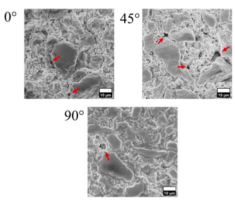
Fig. 17. Cross-section of parts of the HA scaffolds (X, Y plane) printed at three different orientation degrees. Micropores are remarked by red arrows. (For interpretation of the references to colour in this figure legend, the reader is referred to the Web version of this article.)
