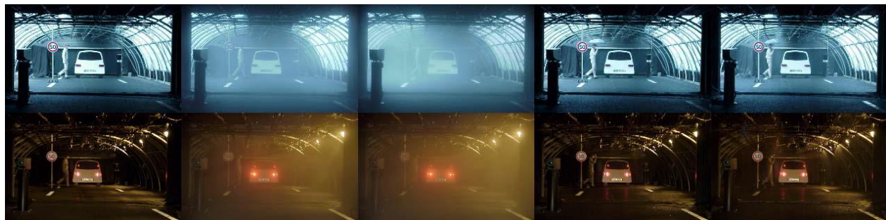
Figure 6 - A selection of images from the Cerema Adverse Weather Pedestrian (AWP) database under different conditions. Top = Day conditions and Bottom = night conditions. From left to right: Normal conditions, Light fog, Heavy fog, Light rain, and Heavy rain. From Dahmane et al. [4].
