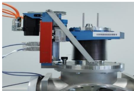
FIG. 2. Allison type emittance meter designed and constructed between 2018 and 2020 by IPHC and institutional partners, commissioned beginning 2021. On the left, the actuator composed of a driving motor, the guiding system and the feedings. On the right, the stainless-steel bellows and the flanges.
