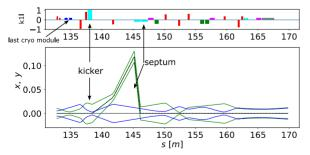
Figure 7: The upper plot shows the element strengths, while the lower one shows the  $6\sigma$  transverse beam sizes starting in front of the last cryo module up to the PTF target.
