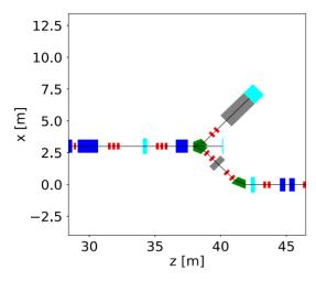
Figure 3: The updated layout of the 17 MeV section between the normal conducting injector (last CH-cavity at z=30m) and the start of the superconducting linac (first two cavities at z = 45 m): RF cavities in blue, dipoles in green, quadrupoles in red, beam dump and vacuum valves in turquois, and shielding wall in grey.
