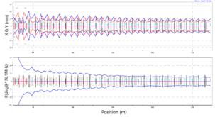
Figure 5:  $6\sigma$  transverse and longitudinal beam size and phase extension (phase relative to the 176 MHz injector frequency).
