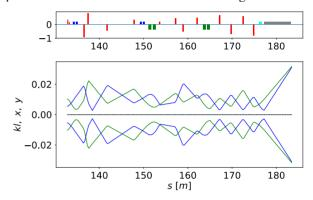
Figure 8: The  $6\sigma$  beam sizes of the beamline towards the FPF facility. The target is located after a 6m shielding wall indicated by the grey box in the upper sub-figure. The two turquois boxes in front of it indicate the two rastering magnets.
