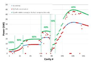
Figure 6: Simulated RF-power needs for: nominal beam operation (blue), a representative case with several failing cavities (red), and the overall expected RF-overhead need to apply failure compensation (green).
