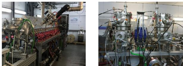
Figure 2: The Injector test stand featuring an ECR ion source, a LEBT, the RFQ and 2 quarter wave rebunching cavities
