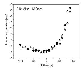
Figure 9: Effect of the high voltage DC bias on the mass variations, while the RF field is kept on at the frequency and power indicated in the inset. Here the device is oriented as in Fig. 2. The voltage has been varied from -1 KVolt to 1 KVolt and backwards, with steps of 100 Volts. The indication of raw mass variation is referred to the fact that data is untreated to compensate any eventual drift.
