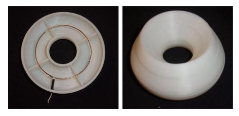
Figure 4: Printed support of the ring (left), relative to the bottom part. The internal copper loop, to be connected to ground through a small radial conductor, is visible. On the right, we can see the two parts assembled.
