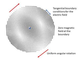
Figure 1: Electric field displacement inside the section of the cylinder at a prescribed time. The picture rotates clockwise with constant angular speed.
