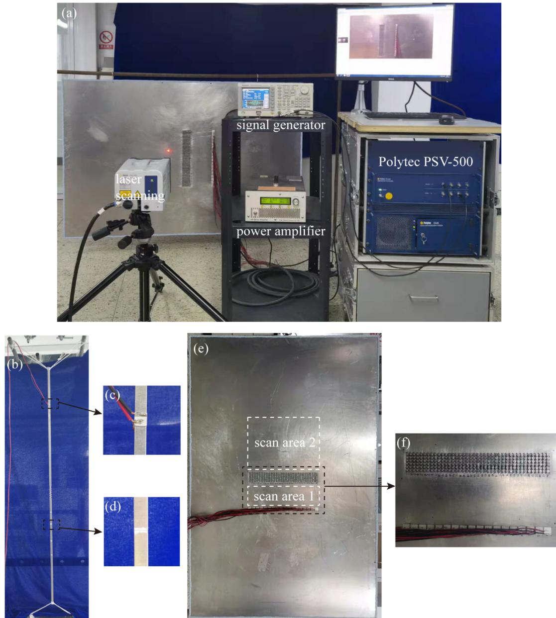
Fig. 3. (a) The experimental setup; (b) the functional element suspended on a vibration isolation table; the zoomed-in diagrams of (c) piezoelectric patch, and (d) measuring line of the phase shift; (e) the manufactured plate; and (f) the zoomed-in diagram of the metasurface structure and piezoelectric patches array.
