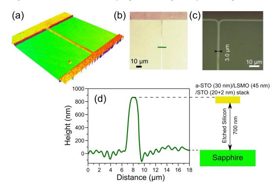
Figure 6: (a) 3D-reconstruction DHM image, (b) 2D DHM image and (c) optical microscope image of a 3  $\mu$ m wide 100  $\mu$ m long suspended bridge; (d) Thickness profile at the position shown in the 2D DHM image of (b) with the schematic cross-section of the suspended a-STO/LSMO/STO stack.
