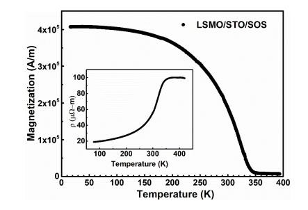
Figure 3: Temperature-dependent magnetization M(T) curve of 30 nm LSMO film on STO buffered SOS substrate, with Tc~340 K. Inset shows temperature-dependent electrical resistivity for the same.
