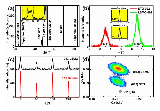
top of STO buffer layer. Whereas, the STO buffer layer tends to relax above a few nanometers thick, as seen from the non-alignment of reciprocal lattice vector position Qx of Si and STO.
