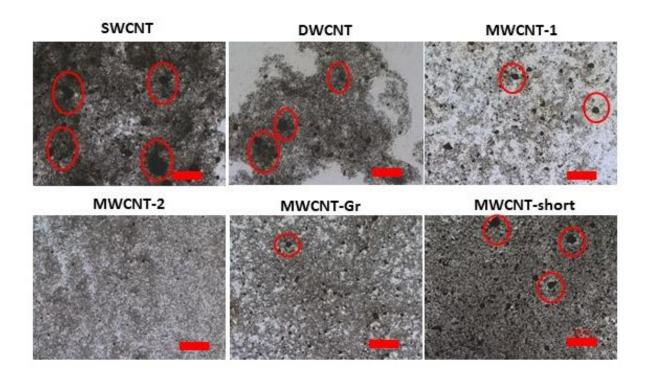
Fig. 3. Optical microscopy images of 0.3 wt% CNT films in diluted PFA resin under the same magnification. Scale bar: 100 μm
