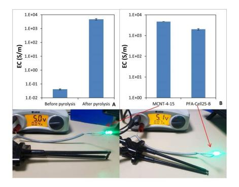
Fig. 12. (A) Electrical conductivity of the composite MCNT-4-15 before and after pyrolysis and
