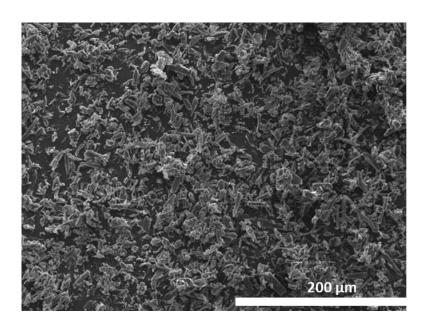
Fig. 1. SEM image of the used cellulose powder.
