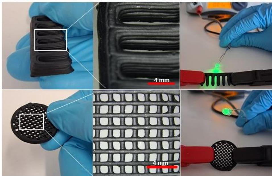
*Fig. 11. Photographs of 3D-Printed objects (left) with microscope zoom (middle) and lighted led lamp using the conductive objects as a link in a simple electrical circuit (right). With connections shown in the images above, the comb-shaped and the cylindrical mesh objects had an electric resistance of 11.7 and 28.7 k $\Omega$ , respectively.*
