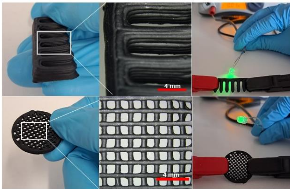
Fig. 11. Photographs of 3D-Printed objects (left) with microscope zoom (middle) and lighted led lamp using the conductive objects as a link in a simple electrical circuit (right). With connections shown in the images above, the comb-shaped and the cylindrical mesh objects had an electric resistance of 11.7 and 28.7 k \Omega , respectively.
