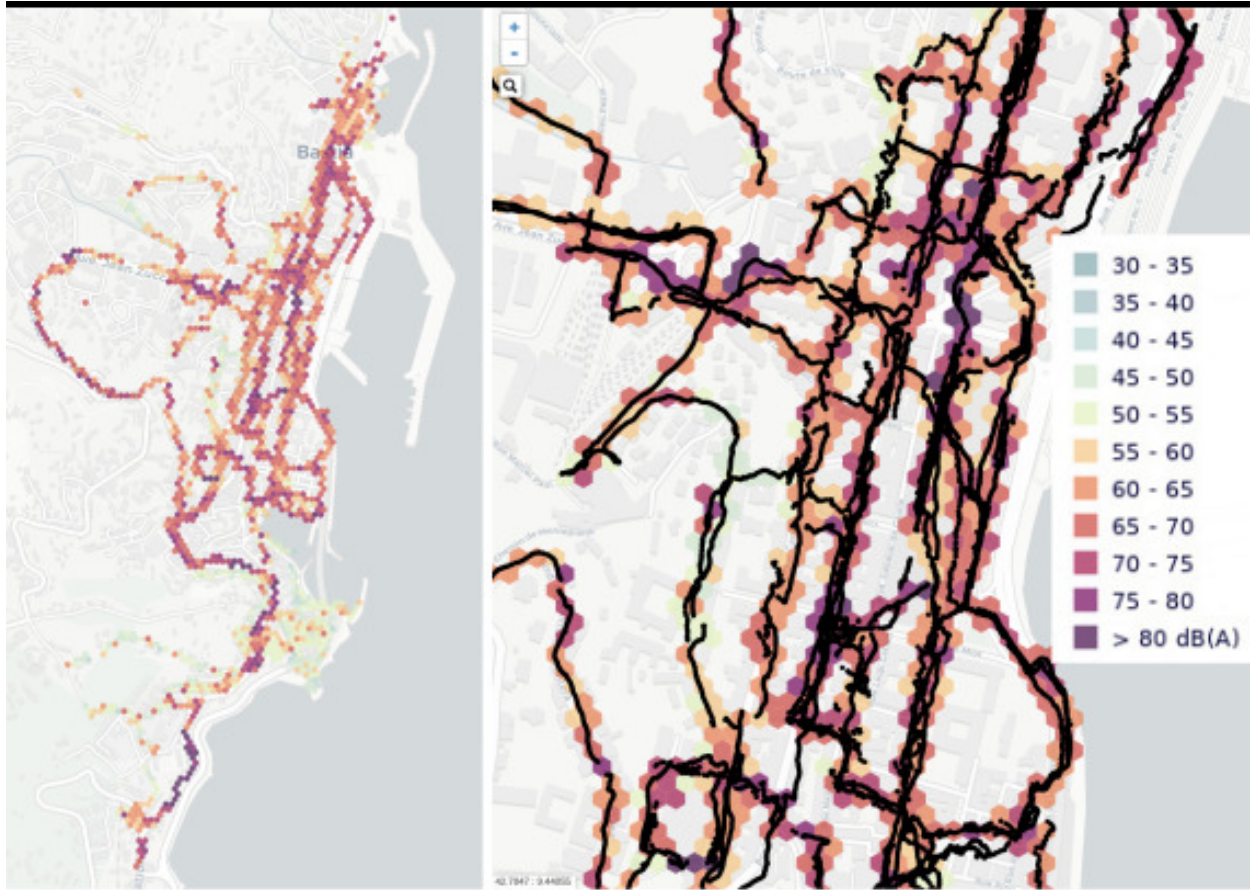
FIG. 9. (color online) Noise map produced (left) on the city of Bastia and (right) downtown zoom with measurement tracks.
