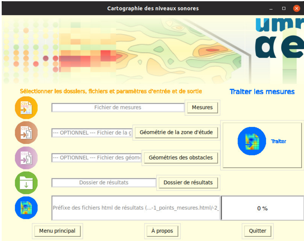
FIG. 6. (color online) Graphical user interface (in french) of the pedagogical toolkit to build a noise map from indoor measurements over a grid of points.
