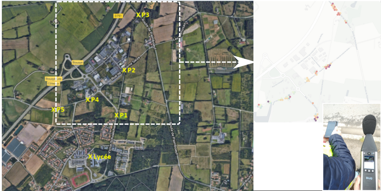
FIG. 2. (color online) Experimental campaign carried out within the framework of the Research Passport operation: (left) location of measurement points, (top right) resulting map and (bottom right) comparison of smartphone measurements with sonometer results.
