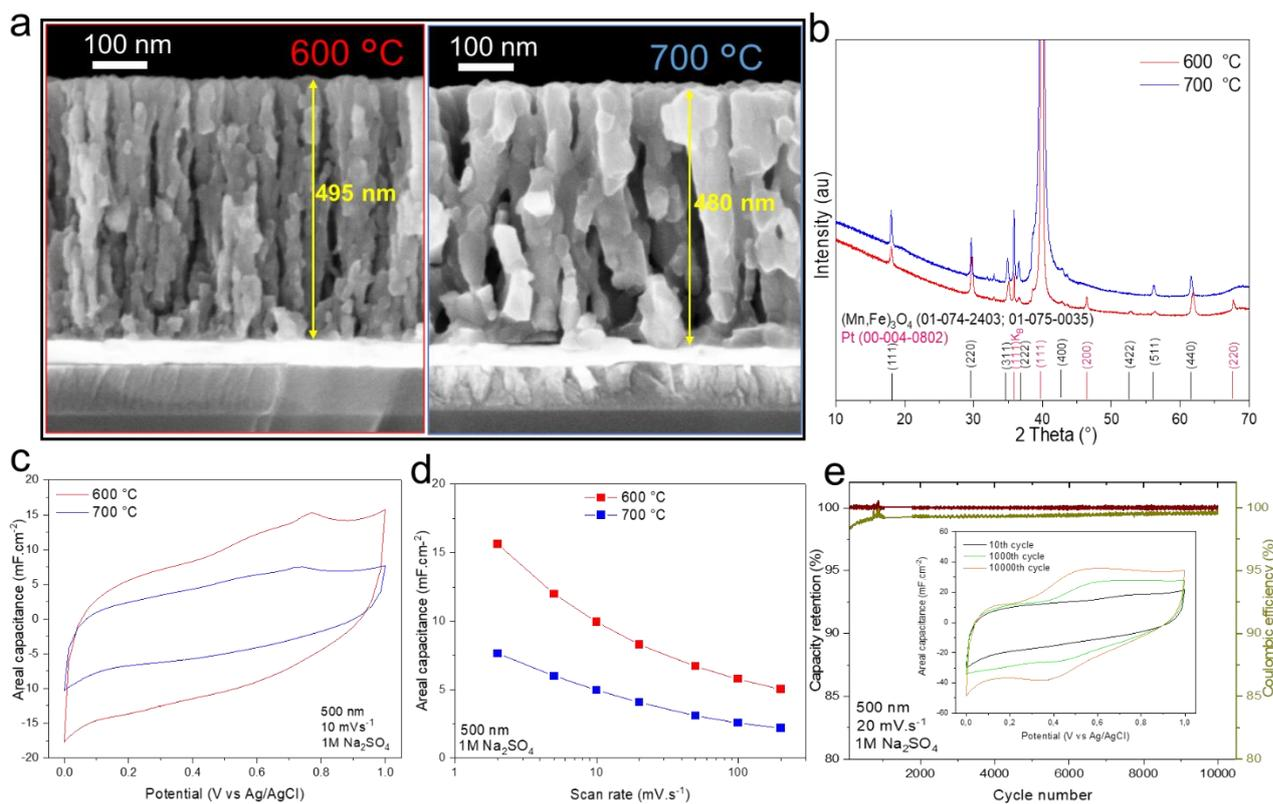
**Fig. 3 | Optimization of post-deposition annealing temperature.** **a.** SEM cross section images of Mn-Fe films (500 nm thick) annealed at 600 °C and 700 °C. **b.** XRD diffractograms of the films. **c.** CV plots of the films at 10 mV.s<sup>-1</sup>. **d.** Evolution of the areal capacitance at different scan rates as the function of temperature. **e.** Capacity retention and coulombic efficiency as a function of the cycle number (inset, CVs of the 10th and 10 000th cycles).
