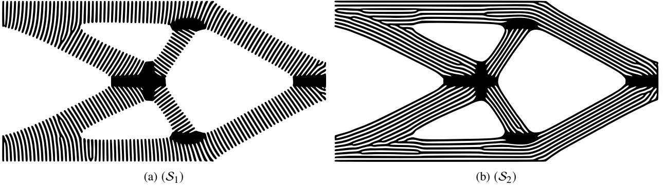
Figure 11: Stress oriented structures for the cantilever 2D generated on 1280 \times 640 mesh, iso at 0.7
