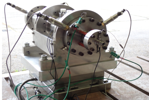
Figure 5: View of the catalytic chamber and the thermocouples mounted on the HYCAT engine.
